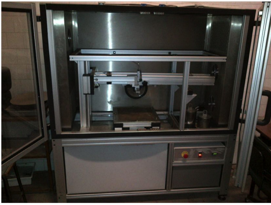
Fig. 2. Wheel Tracker Machine used in DICAM's laboratory.
