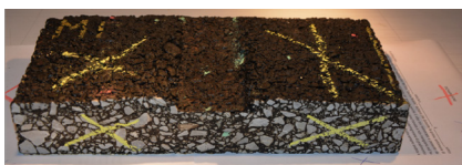
Fig. 3. Rutted sample and marker application.
