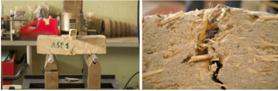
Fig. 68.7 The ASP sample to be tested for flexural strength
