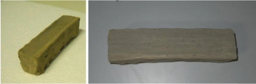
Fig. 68.11 The ASN sample to be tested for abrasion resistance
