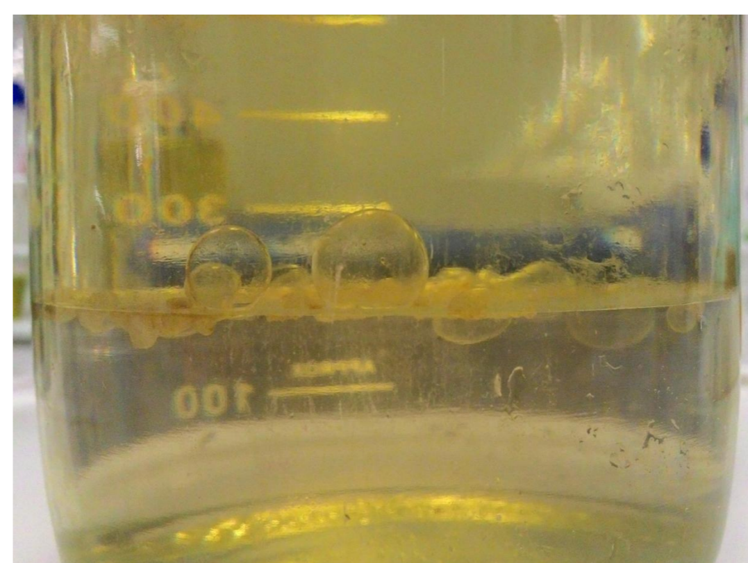
Fig.7 Sample with clear phase separation, up hydrocarbons, down water
