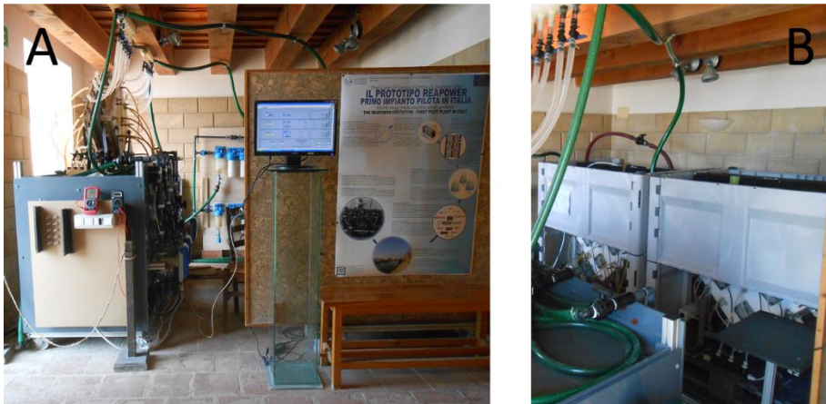
Figure 6.5. Final view of the REAPower demonstration plant. A) The small prototype (44x44 cm 2 , 125 cell pairs) is visible on the left, on the supporting tray. B) Large prototypes (44x44 cm 2 , 500 cell pairs) installed within PP boxes.
