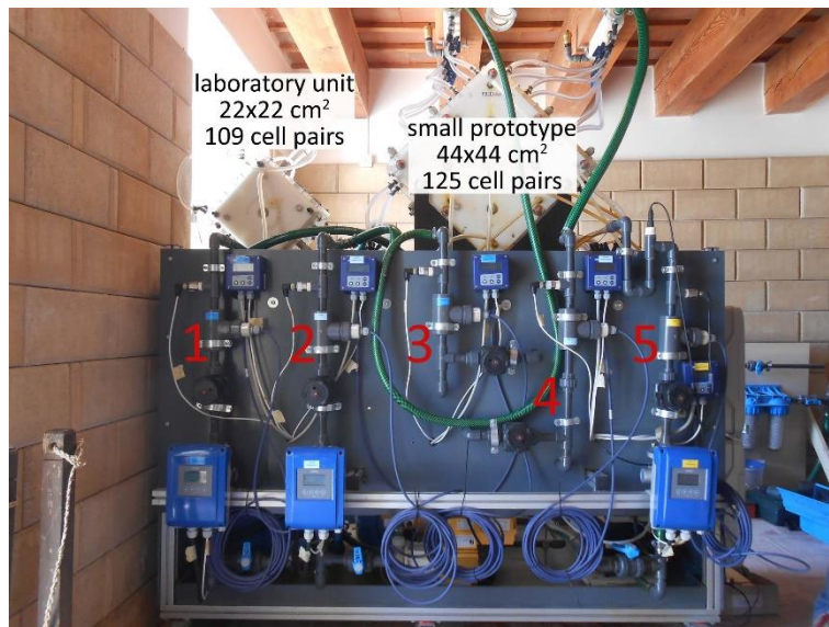
Figure 6.4. Front-end panel of the supporting tray. Five pipelines can be identified: HIGH inlet (1), LOW inlet (2), HIGH outlet (3), LOW outlet (4), ERS (5). A laboratory unit (22x22 cm 2 , 109 cell pairs) and the small prototype (44x44 cm 2 , 125 cell pairs) are shown on the tray.
