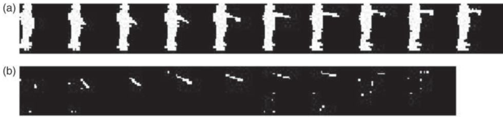
Figure 5. (a) The sequence of images depicting the check watch action and (b) the sequence of images obtained by subtracting consecutive images of the check watch action.
