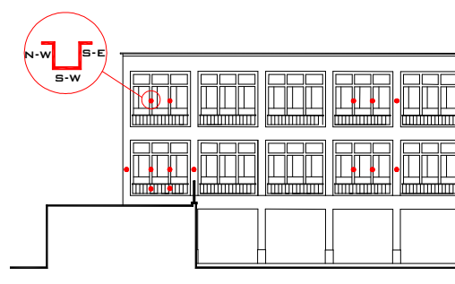
Figure 6. Department of Hydraulics South-West façade, with monitored points in red and the cross-section of a pillar, with different exposures
