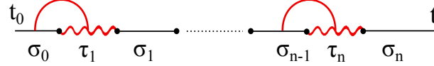
Figure 3.6: Interactions retained in the extended-NIBA: intra-blip interactions (red wavy lines) and blip-preceding sojourn interactions (red semicircles). Example of a TLS path of n transitions.
