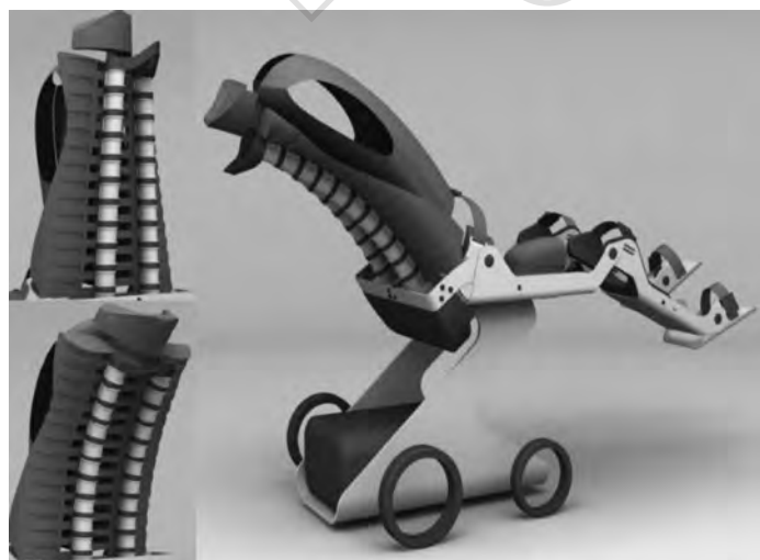
Figure 1.—Electronically controlled dynamic backrest.
