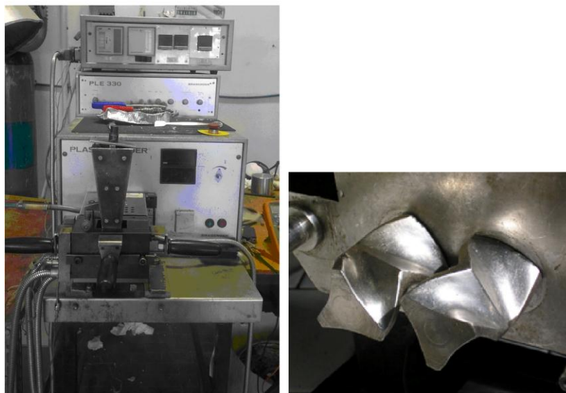
Figure 3.1) Discontinuous internal mixer (brabender) and its twin screws
