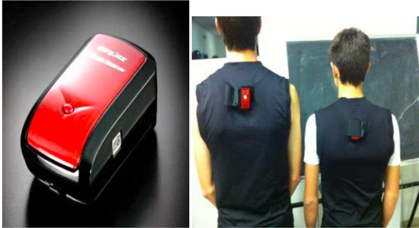
Fig 13 – GPS (Global Positioning System) QSTARZ 10Hz
