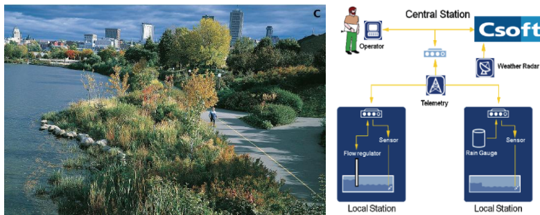
Figure 3.4: The St-Charles retention basin and the architecture of the RTC system implemented in Quebec City.
