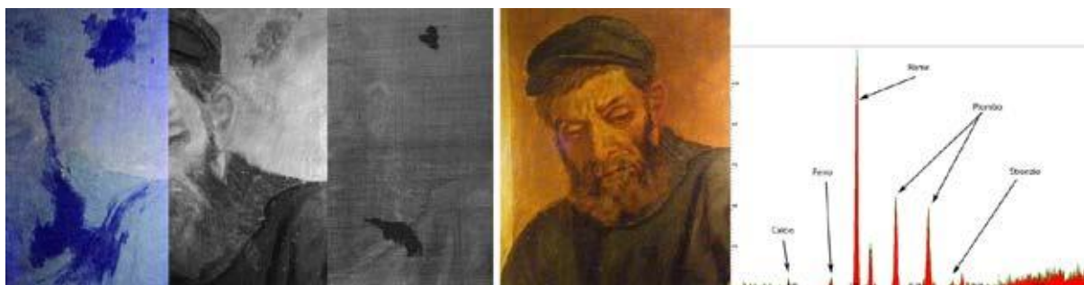
Figure 1: Application of multispectral imaging and XRF spectroscopy on a painting on canvas
