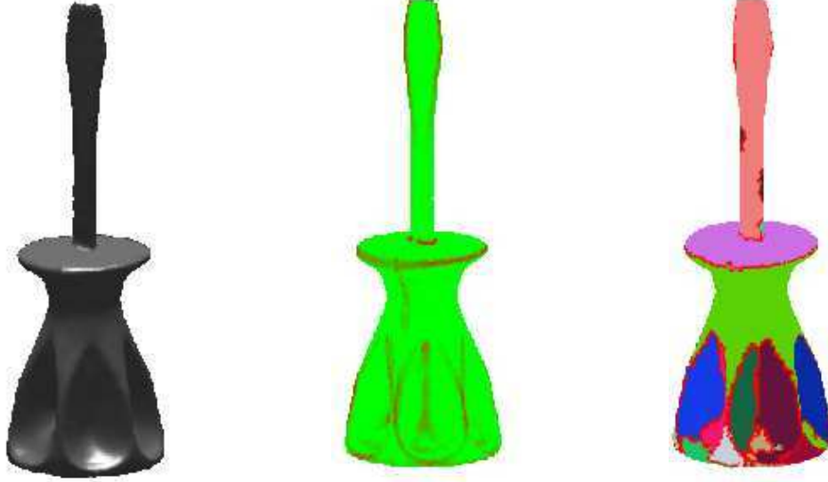
Figure 4.11: Original screwdriver object ( left ). Feature-edges detected by SCD ( middle ). Watershed segmentation ( right ).
