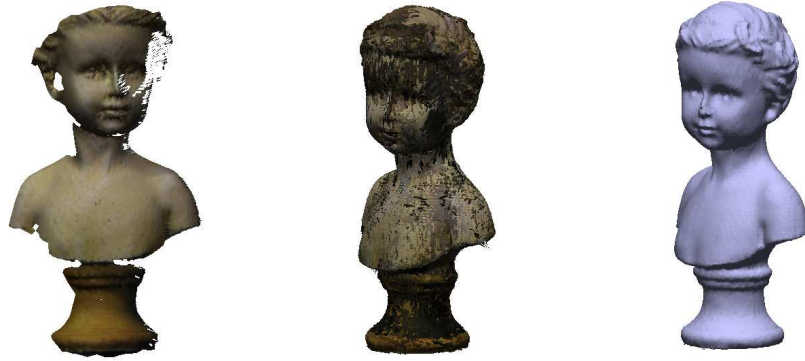
Figure 1.2: Two range images ( left and center ) representing two different points of view of a sculpture, with the reconstructed shape ( right )
