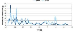
Fig. 9: accelerations in the side crash at 40 km/h
