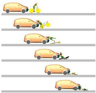
Fig. 11: telescoping at constant speed 20km/h.
