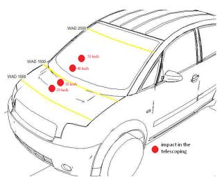
Fig. 22: head contact points in the telescoping.
