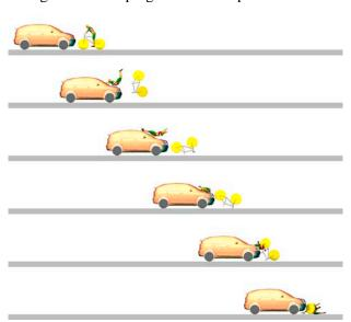
Fig. 12: frontal crash at constant speed 30km/h.
