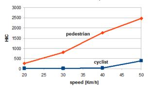
Fig. 15: comparison HIC teenage cyclist – teenage pedestrian in frontal crash [1].
