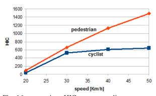
Fig. 16: comparison HIC teenage cyclist – teenage pedestrian in side crash [1].
