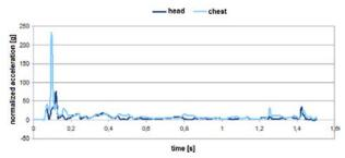
Fig. 8: accelerations in the frontal crash at 50 km/h
