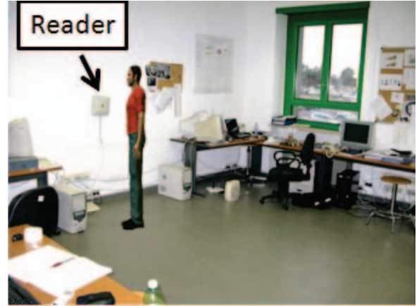
Figure 2. Experimental setup. The volunteer equipped with a wearable tag walks away from the reader's antenna which is placed onto the wall of a 5.5m \times 5.5m \times 3m room, at 1.3m from the floor. The experiment is repeated for four orientations of the body with respect to the reader's antenna, e.g. for \phi_n = 0, 90, 180, 270 degrees.
