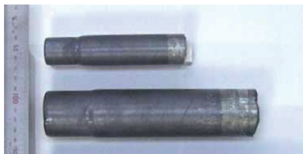
Figure 14 CdTe single crystals, grown by using the THM technology. Courteously provided by Acrorad (Japan).
