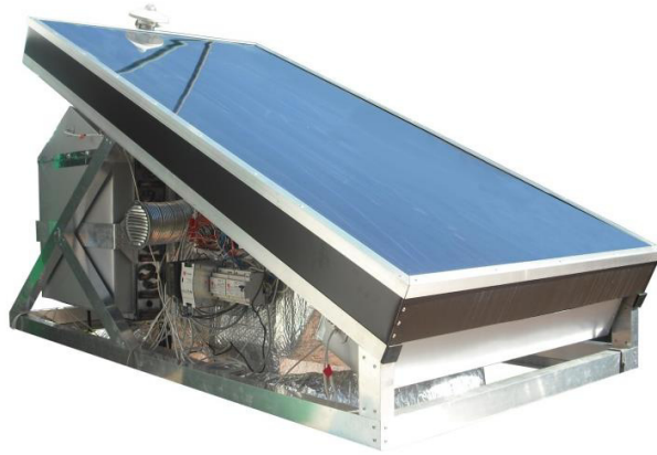
Fig. 3. Picture of the prototype of the solar air conditioner
