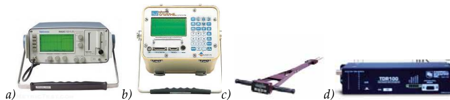
Figura 2.4 - Apparecchi TDR. a) Tektronix 1502C (Tektronix Inc.), TRASE System I (Soil Moisture equipment Corp.), c) Field Scout TDR300 (Spectrum Technologies, Inc), d) TDR100 (Campbell Scientific Inc.)
