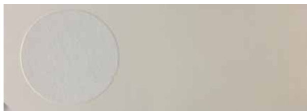
Photograph 1. Circular PTFE swab mounted onto card (real scale).
