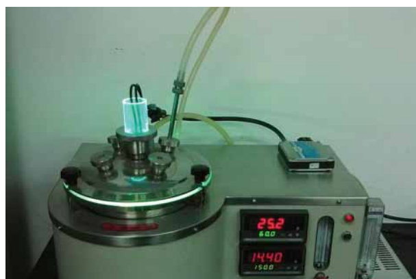
Fig.3 the VOCs collecting apparatus with a the xenon lamp
