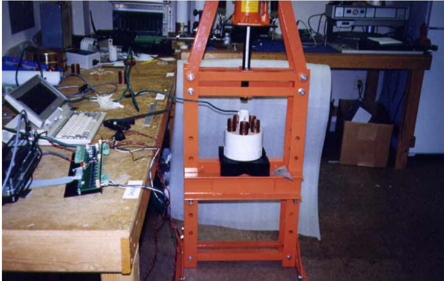
Picture 2B. Details of volumetric soil water content and bulk density sampling (5 small copper rings around the sensor), for laboratory calibration of impedance Hydra Probe(Vitel Inc.) sensor, as reported by Paltineanu, I. C., (2000 – unpublished data)
