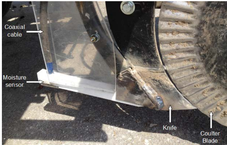
Figure 2. An applicator knife equipped with the prototype soil moisture sensor.
