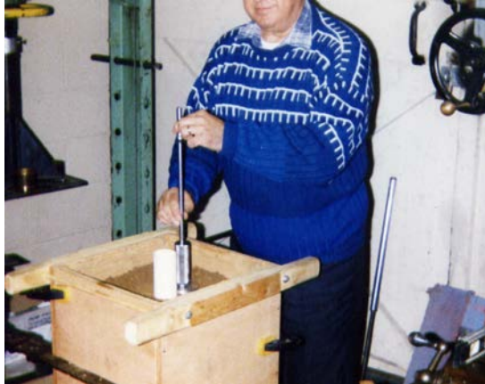
Picture 1. Experimental setup, using a 50 T hydraulic press, and details of volumetric soil water content and bulk density sampling (5 brass rings around the sensor) for laboratory calibration of fringe capacitance probe EnviroSCAN (Sentek Technologies), as reported by Paltineanu and Starr, (1997).
