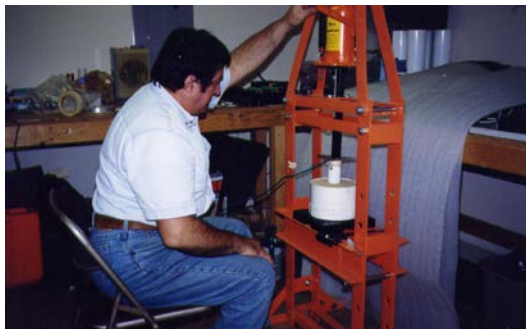
Picture 2A. Experimental setup, using a 20 T hydraulic press, for laboratory calibration of impedance Hydra Probe (Vitel Inc., VA, USA) sensor, as reported by Paltineanu, I. C., (2000- unpublished data).
