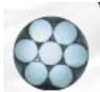
Fig. 26 - Section of a bundle of 7 fibers, six transmitting fibers (two fibers for each LED) were arranged in a ring around a central receiving fiber.
