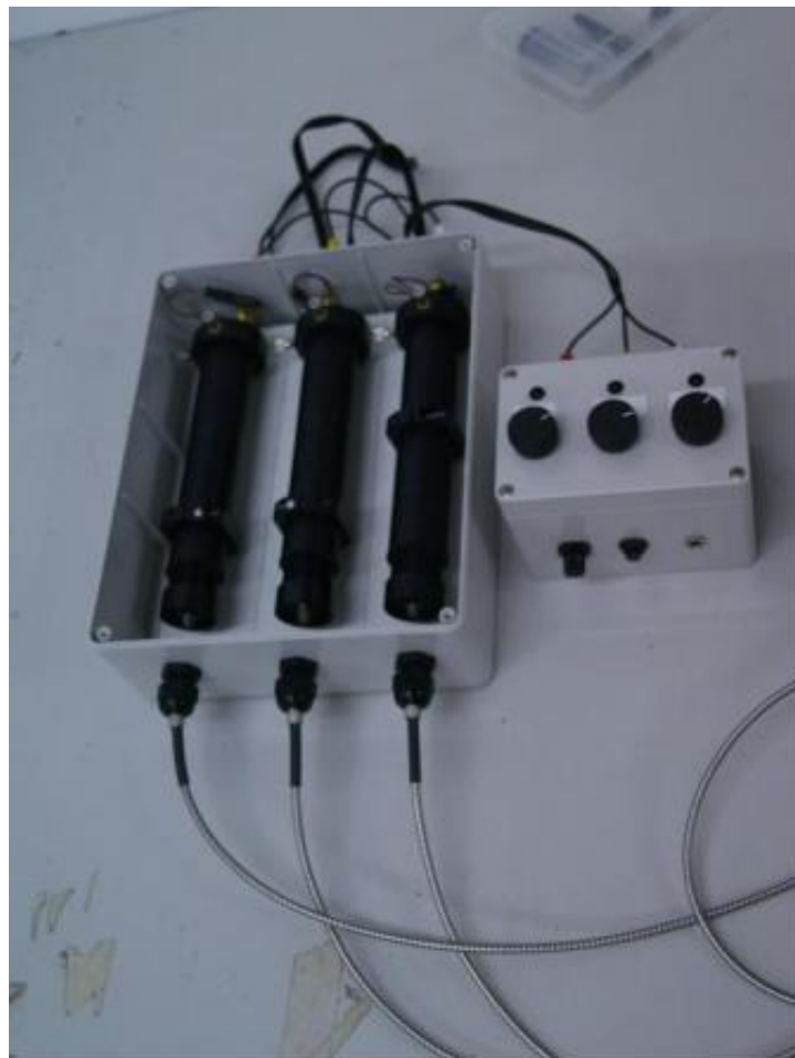
Fig. 29 - Multi-UV-LED light source is composed by three separate optical systems with electronic system for the intensity variation.
