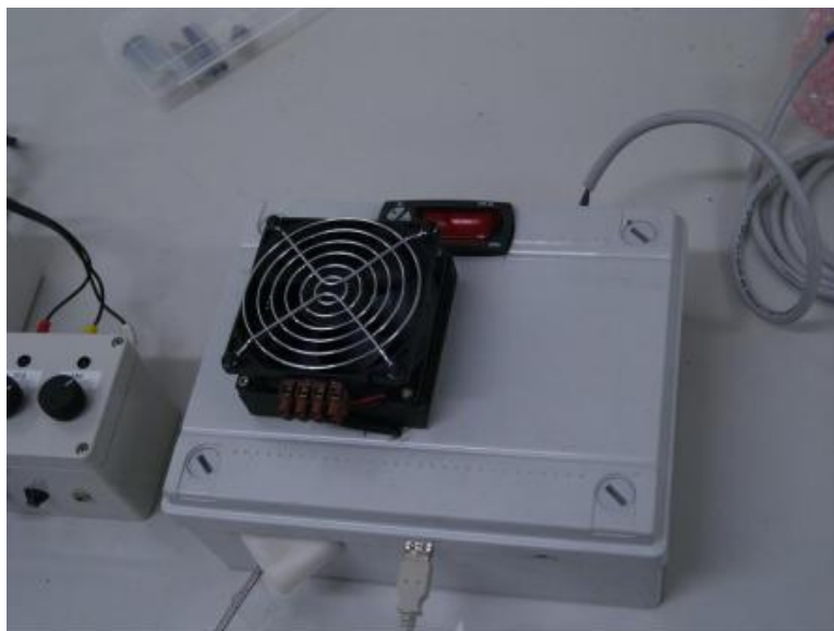
Fig. 32 - Isothermal box whit SuperCool® PR-59 thermoelectric cooling/heating and digital control unit
