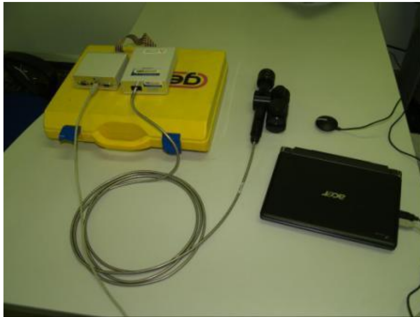
Fig. 52 - Mobile mini-DOAS instrument essentially formed by a telescope a optical fibre, one spectrometer, one GPS, and a PC.
