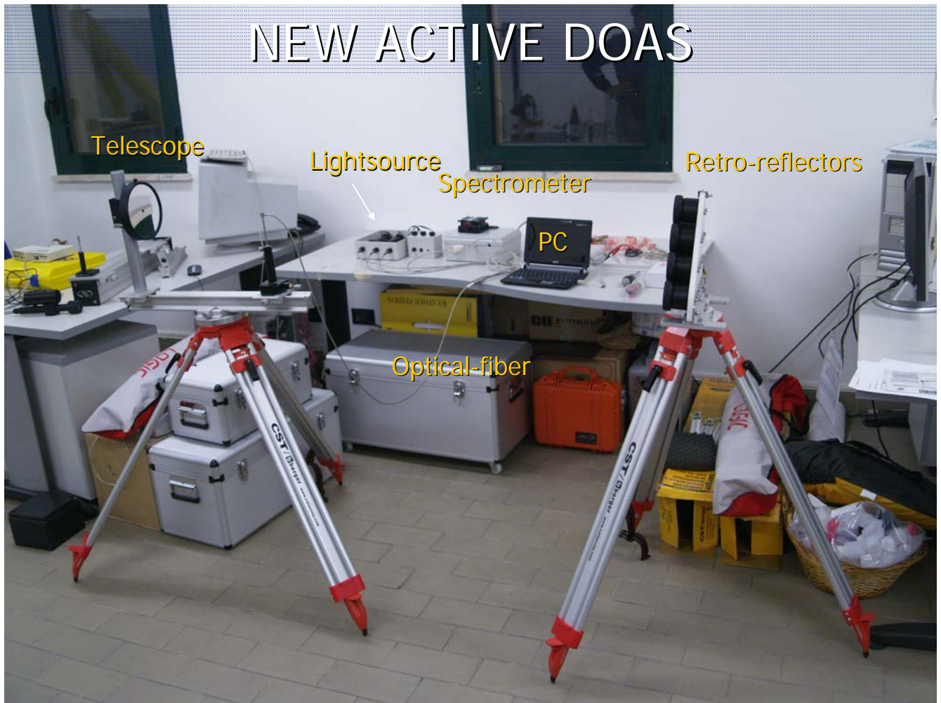
Fig. 24 - NewActive Doas composed by one telescope, a optical fiber, three UV LED sources, one Spectrometer, a retroreflector and one notebook
