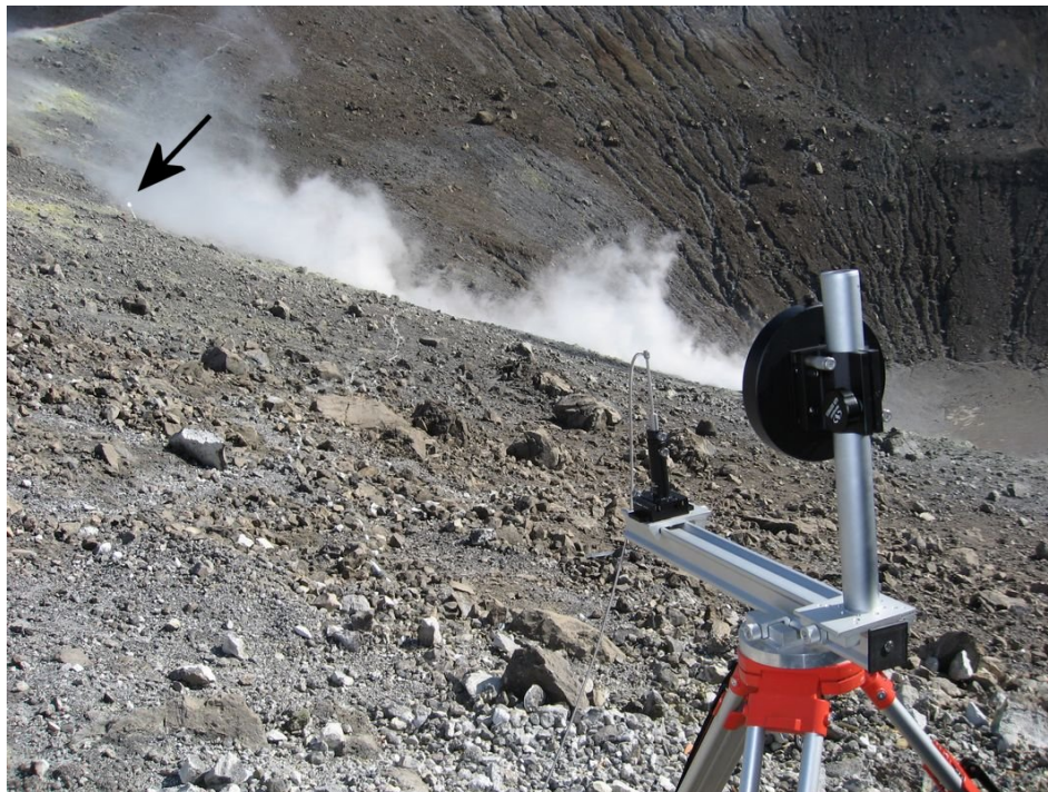
Fig. 39 – The arrow indicated the location of the retro reflector array during the second measurement period on February 25, 2010 (Position 2). The reflectors are now located further down in the crater to enable the measurement of gas being emitted from the high temperature fumaroles in the crater floor.
