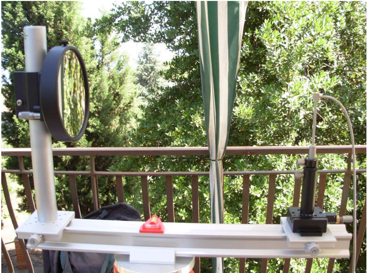
Fig. 25 - Detail of the telescope consists of a Spherical mirror mounted on a special support that allows the movement along the X Y directions. An aluminium optical bench allows the position in line between the mirror and the optical fiber positioner, that allows the movement along the Z direction.
