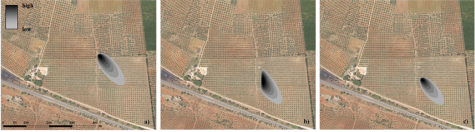
Figure 6.2: Footprints for the installations: a) EC1, b) SAS and c) EC2, calculated using the model of Kormann and Meixner (2001) for the daytime predominant wind direction ( 140^\circ ). The three areas encompass the 90% of the observed fluxes in the unstable conditions defined by u_* = 0.4 \text{ m s}^{-1} and L = -50 \text{ m} .
