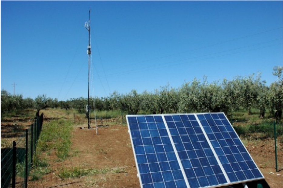
Figure 5.8: Eddy-covariance installation EC1.
