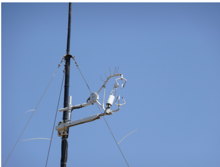
Figure 5.9: Detail of CSAT3-3D sonic anemometer and LI7500 open-path gas analyzer the of the EC1 system.
