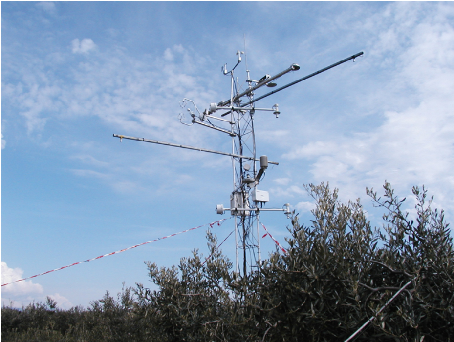
Figure 5.13: Eddy-covariance installation EC2.
