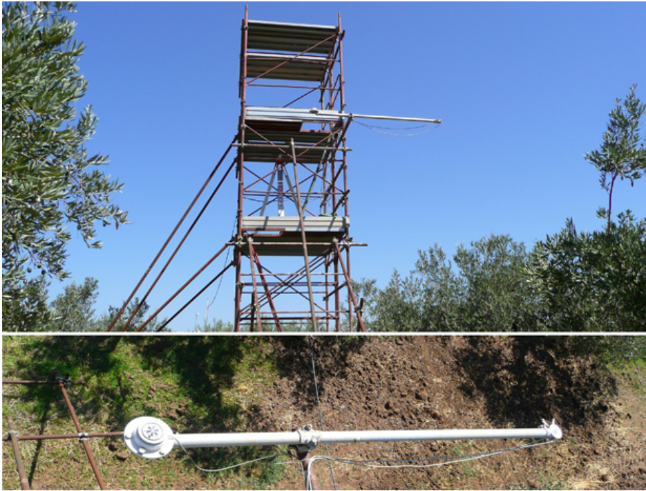
Figure 5.11: Pyrradiometer ( Schenk GmbH , model 8111) of the OEBMS1 system installed on the SAS transmitter iron-frameworks at an elevation of 8 m a.g.l. (upper panel). In the lower panel a detail of the pyrradiometer (on the right side) and of the solar radiometer (on the left side).
