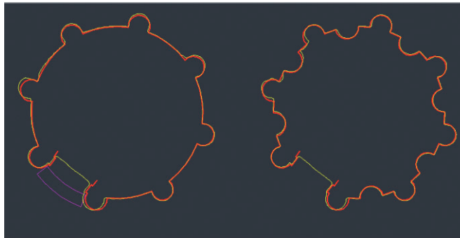
Figure 28: Auteri Chapel reconstruction error evaluation on horizontal profiles: yellow 123D Catch model, red GCP survey
