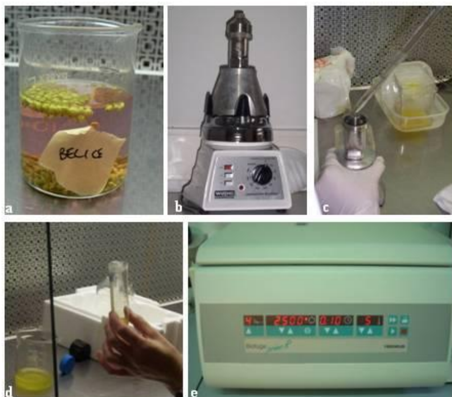
Fig. 2.1 Microspore isolation protocol: (a) sterilization of flower buds with 70% ethanol solution; (b) blender; (c) washing with mannitol solution; (d) re-suspending of microspore pellet; (e) Prime R centrifuge (Biofuge, Heraeus).
