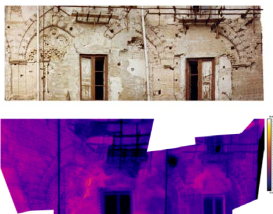
Figure 1. Palermo, Diana di Cefalà palace, photogrammetric survey of the façade and mosaic of thermograms partially distorted
