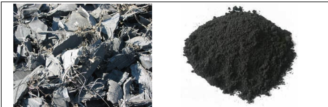
Figure 4.15b. Shredded tyre (left) and crumb rubber (right)
