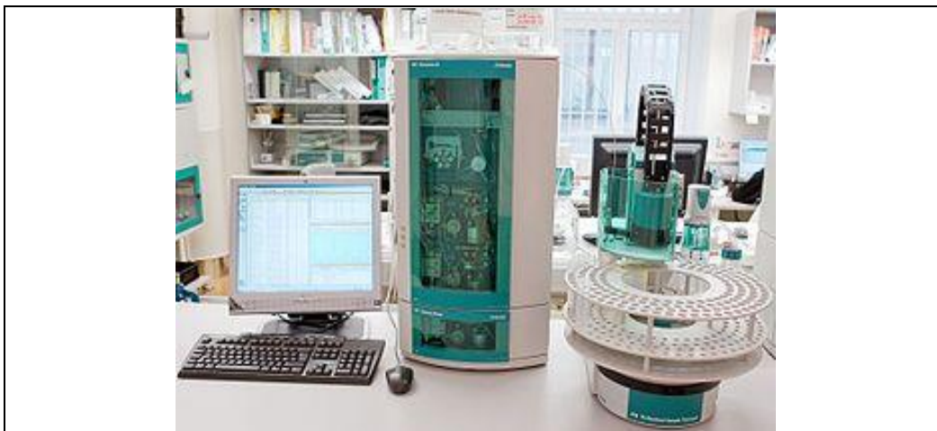
Figure. 2.5. Example of IEC equipment
