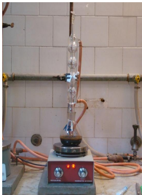
A - condensation column
