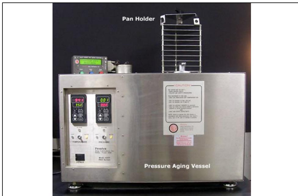
Figure 3.10. PAV equipment (PavementInteractive.org, 2010).
