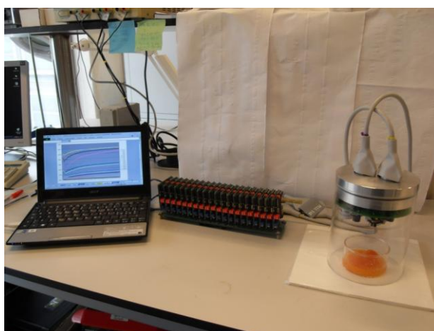
Fig. 6.1.c E-nose IQMA with joint concentration and measure chambers.
