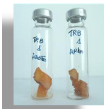
Fig. 4.3.a Electronic nose samples: vials sealed in atmosphere air (R) or saturated of nitrogen (L).
