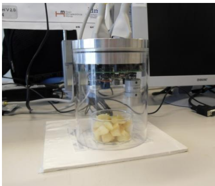
Fig. 6.2.b E-nose IQMA with joint concentration and measure chambers.
