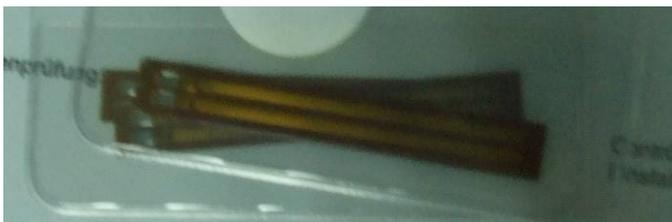
**Fig. 2-7 - Strain Gauges HBM LY41 50/120**
