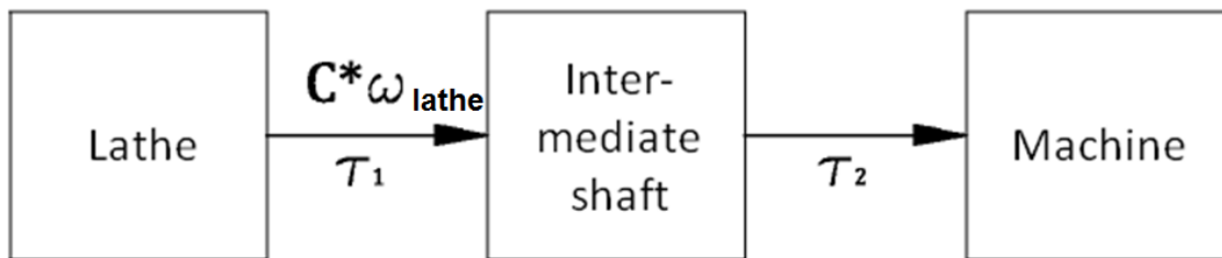
Figure 35. block diagram of the machine kinematic chain
