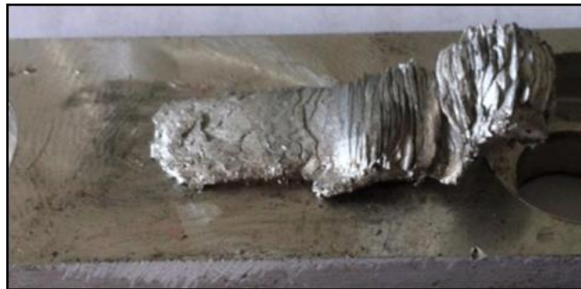
Figure 109. Instability effect, 57.8 Hz, 40 MPa
