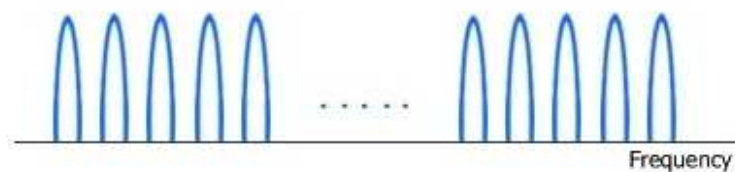
Figure 1: Placement of subcarriers in FDM.
