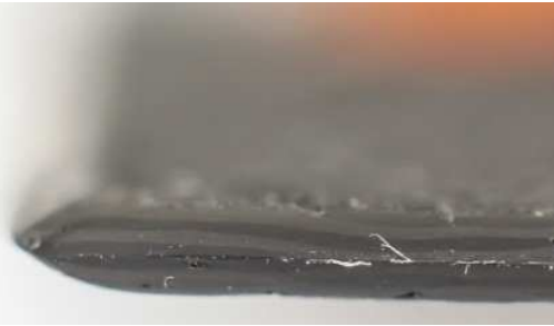
Figure 4: Edge detail of the specimens used for tensile test (transverse section).
