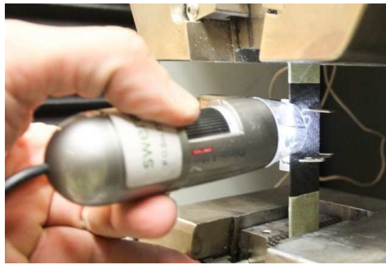
Figure 6: Analysis of damage mechanism under tensile load by using Dino-Lite Pro microscope.
