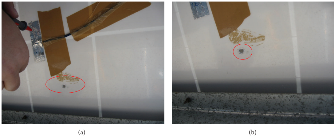
FIGURE 9: Experimental apparatus: little holes in the PET film of the PV panel to measure the temperature.
