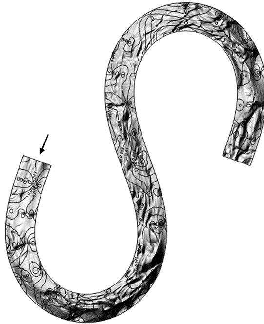
Figure 8. Comparison between the DSM and the contour-lines of shear flow velocity, u_* (m/s), along the channel reach between sections 7 and 31
