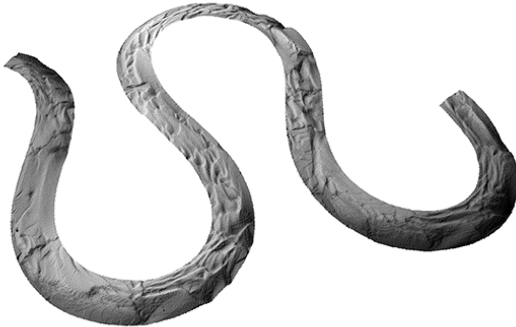
Figure 4. 3D view of the DSM of the meandering channel
