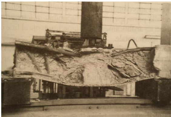
Figure 2.13. Specimen at the end of the test with no spalling of the concrete thanks to the presence of the inferior steel plate.
