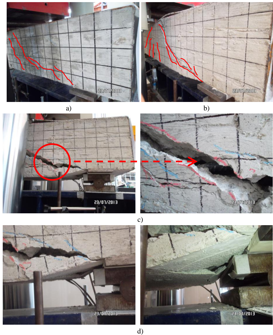
Figure 5.33. Specimen B1: a) appearance of the diagonal cracking; b) growing of the diagonal shear crack; c) dowel mechanism; d) local crushing of the concrete at the support.
