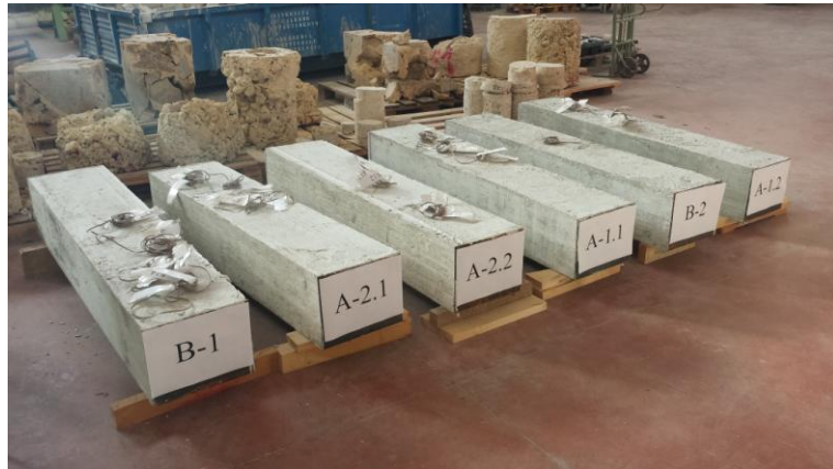
Figure 5.5. Specimens after the concrete casting.
