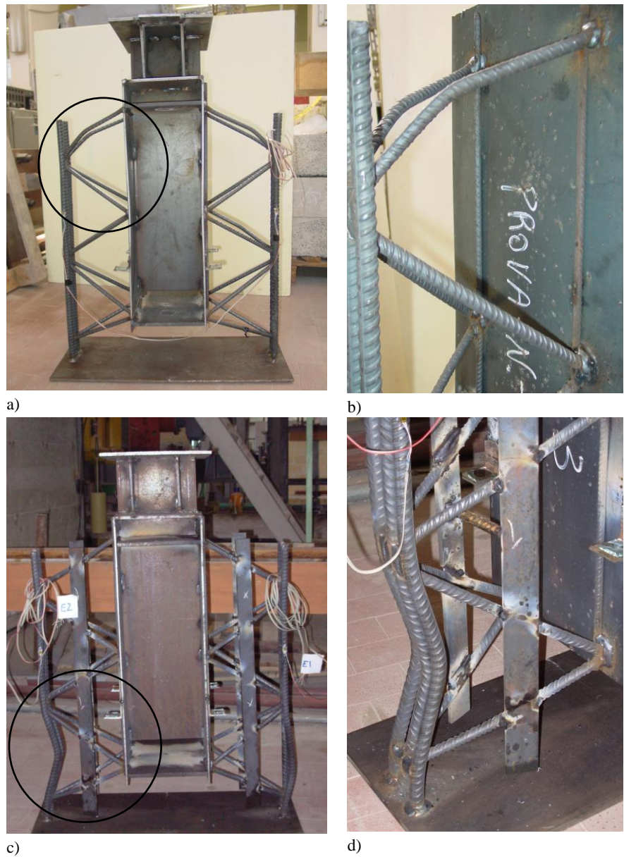
Figure 7.4. Specimens of push-out tests in phase I at the end of the test: a) specimen S1; b) zoom of web bars in specimen S1; c) specimen S2; d) zoom of upper chord in specimen S2.
