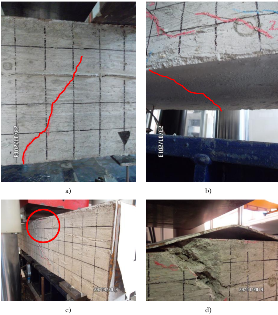
Figure 5.32. Specimen B1: a) flexural cracks; b) cracking of the face opposite to the steel plate; c) buckling of the compressed plate in the initial phase; d) buckling of the compressed plate at the end of the test.
