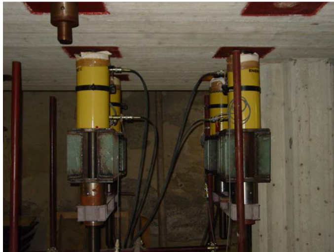
Fig. 2.6. Hollow hydraulic jacks for vertical load application.
