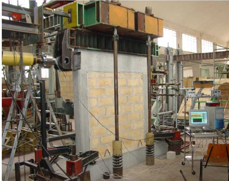
Fig. 2.10. Calcarenite masonry infilled frame specimen in the test apparatus.
