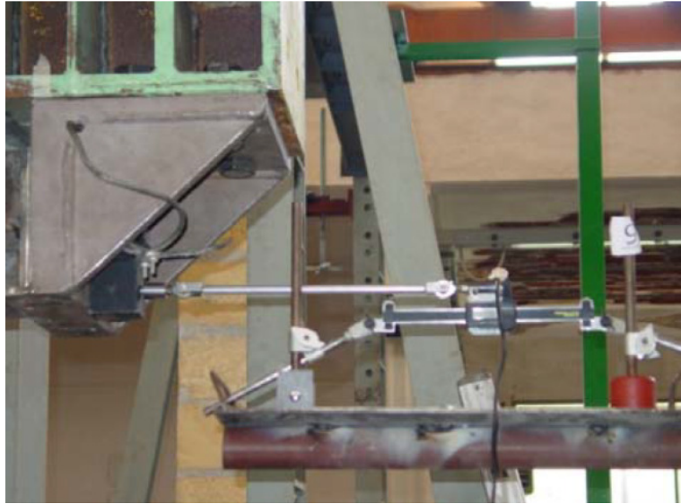
Fig. 2.9. Gauge for the top lateral displacement measuring.
