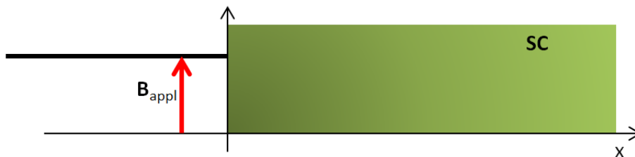
Figure 11.3.: Section of the superconductor, in green. The red arrow represents the magnetic field applied parallel to the surface.
