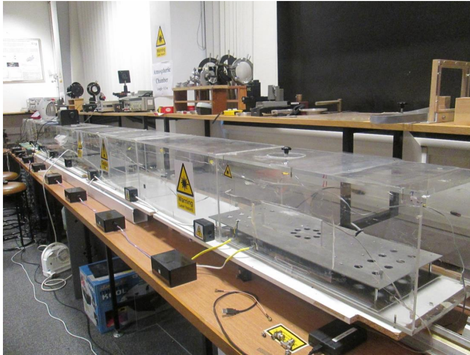
Figure 3.5 – Indoor atmospheric chamber – Optical Laboratory of Northumbria University.
