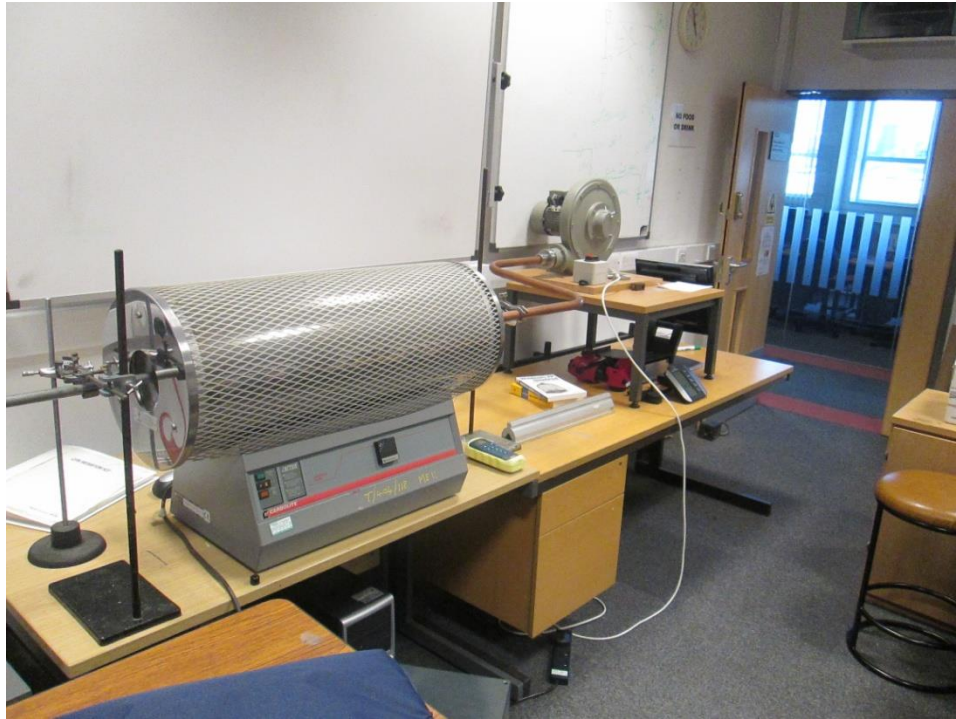
Figure 3.6 – FSO channel composed by a temperature-controlled oven and an air pump.
