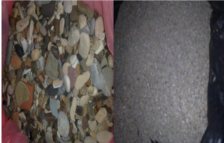
Figure 4.4. Fine sand and large gravel used in the BSF
