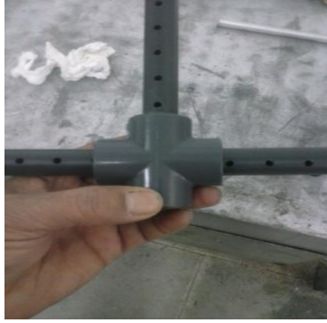
Figure 4.5 The used inlet water diffuser
