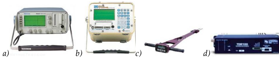
Figura 1.10 Apparecchi TDR. a) Tektronix 1502C (Tektronix Inc.), TRASE System I (Soil Moisture equipment Corp.), c) Field Scout TDR300 (Spectrum Tec., Inc), d) TDR100 (Campbell Scientific Inc.)
