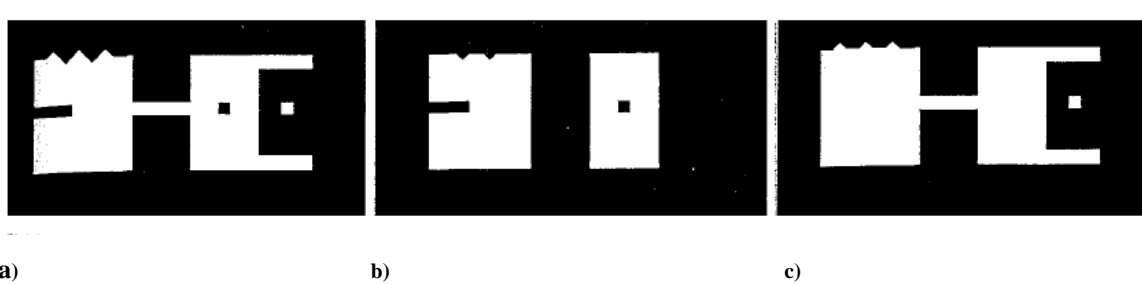
Figure B.3: a) Original image; b) Opening of a; c) Closing of a
