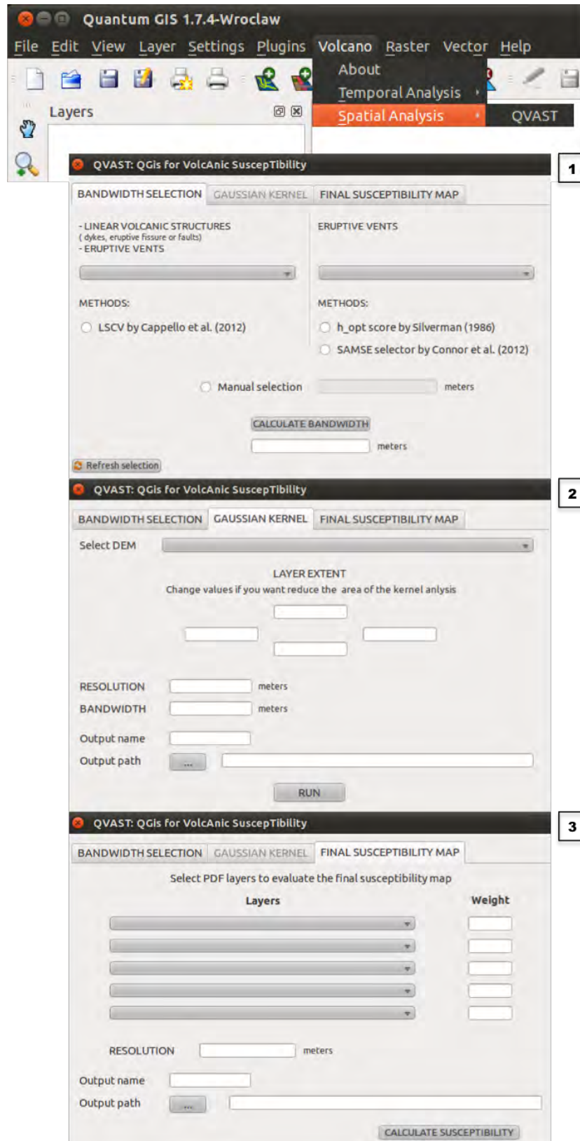
FIGURE 2: QVAST main interface: screenshots for the optimal bandwidth selection (1), for the parameter needed by the Gaussian kernel (2) and for the assignment of weights to the different PDFs (3)
