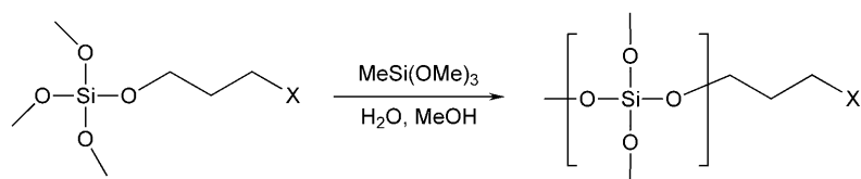
Scheme 1. Organically modified silica are sol-gel hybrid organic-inorganic material. Sol-gel process: hydrolysis and co-polycondensation.
