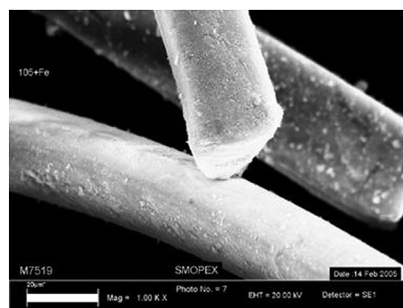
Figure 5. FibreCat fibers under the scanning electron microscope [Reproduced from Ref. [39], with kind permission]. Scale bar represents 20 \mu\text{m} .
