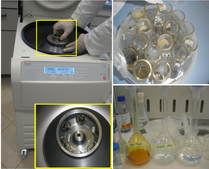
Figure 19: Centrifuge, extractant and other tools used for SEP procedure.
