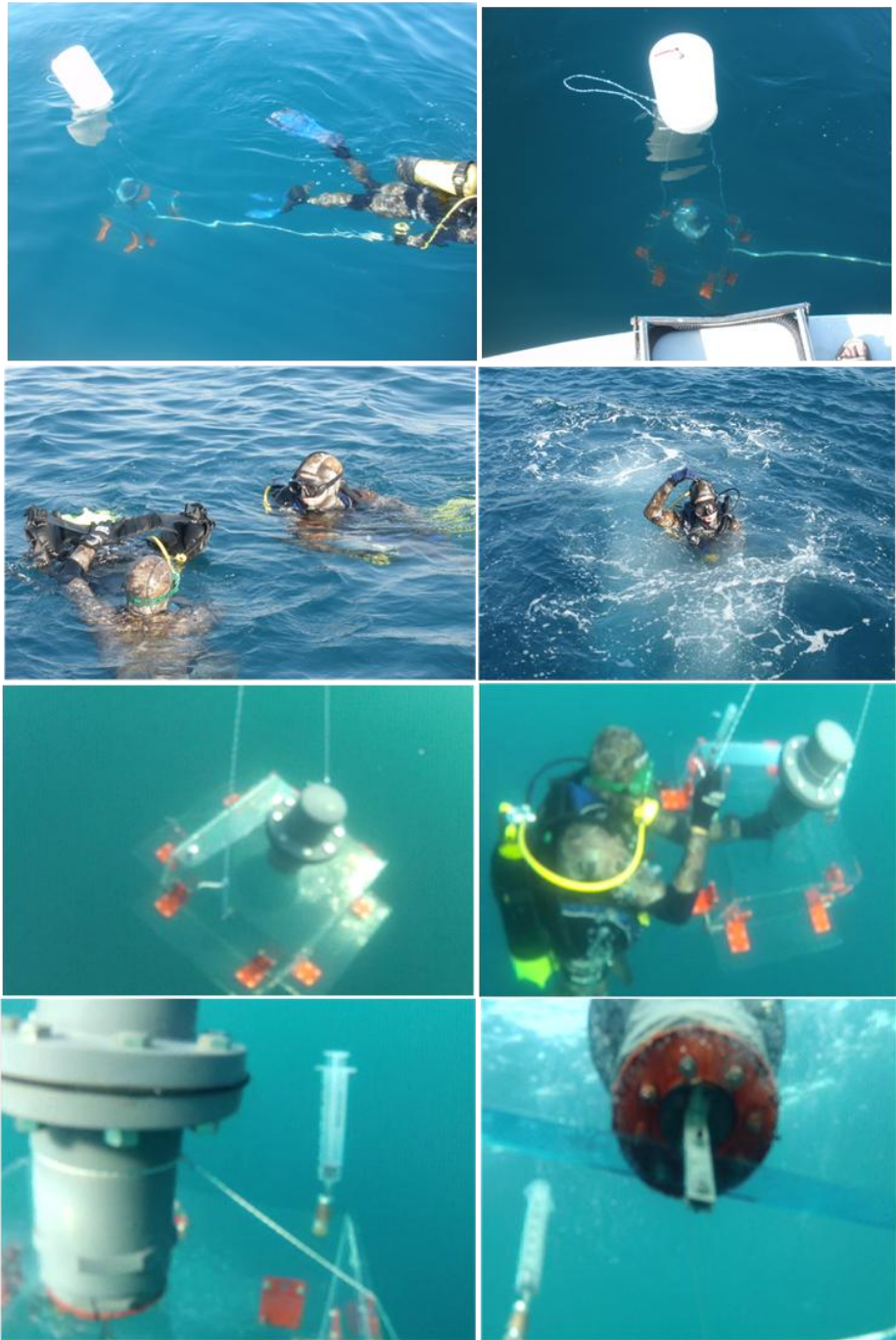
Figure 16: Sub aerial and submarine imagines of benthic chamber setting in the bottom sediment by scuba diver (photo of V. Di Stefano and C. Patti).
