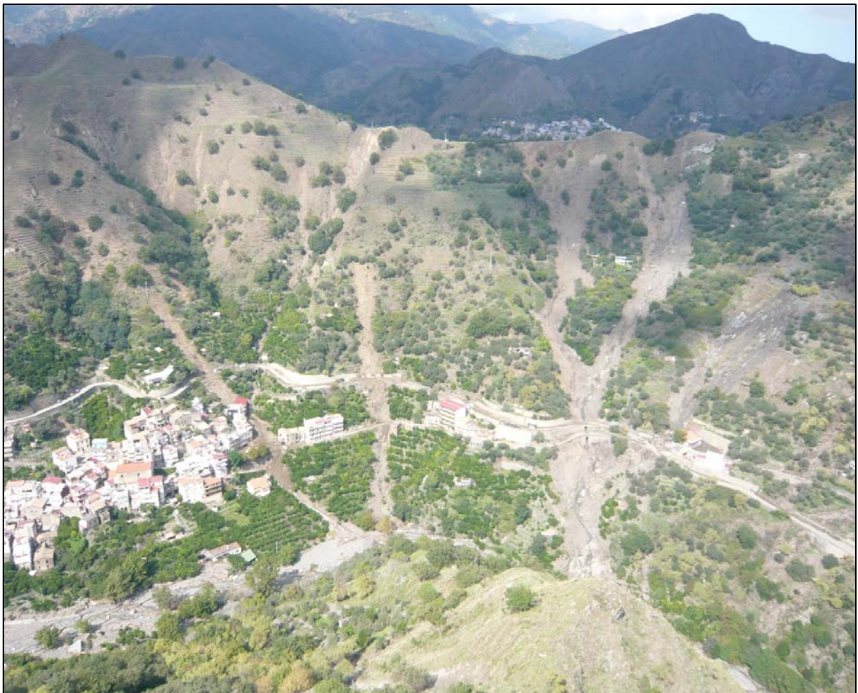
Fig. 2.17 – Overview of a slope affected by the rapid development of multiple debris flows coalesced, triggered during flood event that hit the town of Altolia (Me) in 2009. The material in question coincides with the layer of loose material. These materials are often placed on very steep slopes and in poor stability, in association with intense weather events, dangerous flows of feed with a high destructive power.
