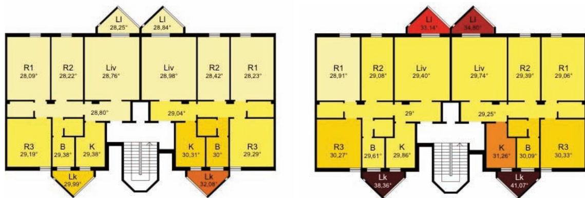
Fig. 25 - Thermal map of the typical right and left apartments on August 15th at 6AM (left) and at 4PM (right) for the current state
