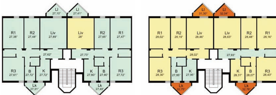
Fig. 27 - Thermal map of the typical right and left apartments on August 15th at 6AM (left) and at 4PM (right) for the scenario with outside vegetation
