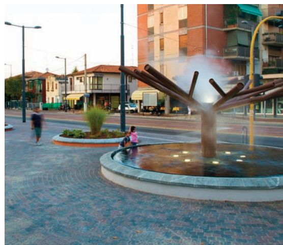
Photo 1 and 2 - Two example of evaporative cooling strategie: systems of fountains in the XII cent. arab building “La Zisa” in Palermo (left) and nebulizers installed in a square in Padua, Italy (right)
