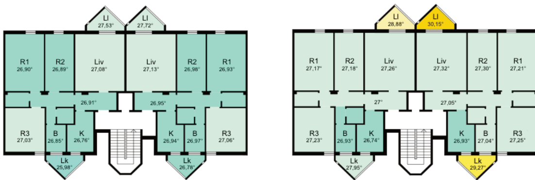
Fig. 29 - Thermal map of the typical right and left apartments on August 15th at 6AM (on the left) and at 4PM (on the right) for the scenario with silver low-e glazing windows and living walls
