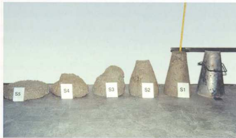
Figure 3.10-Samples of different consistency classes and Abrams cone
