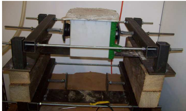
Figure 4.32 Horizontal steel Frame for ultrasonic test
