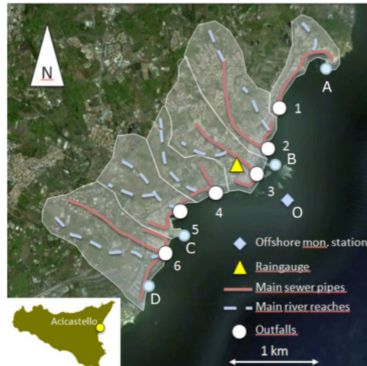
Figure 1: The analysed area: the station O collects hydrodynamic data and water quality samples; stations A, B, C and D collect water quality samples only.
