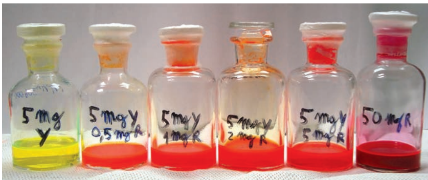
Figure 7. Color palette obtained mixing different concentrations of yellow and red dyes in the PMMA solution. From left to right, concentrations of yellow and red dyes in PMMA have the following pairs of values (mg/mL of Lumogen Yellow; mg/mL of Lumogen Red): (5; 0), (5; 0.5), (5; 1), (5; 2), (5; 5), (0; 50).
