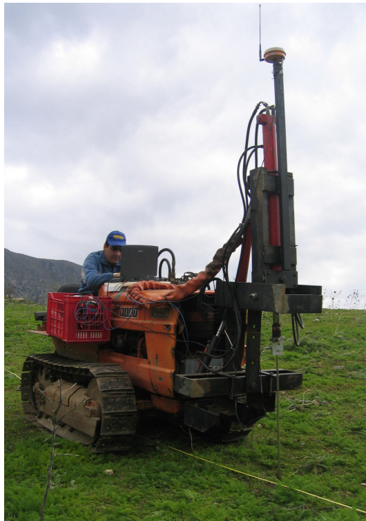
"Figure 1 – The system for measuring the geo-referenced soil cone penetrometer resistance."
