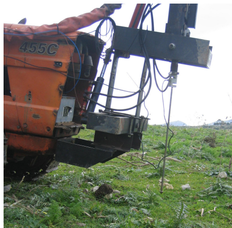
"Figure 2 – Tekkal ABA 300 load cell, connected to the penetration rod and cone."
