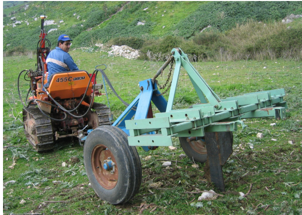
"Figure 3 – The system for measuring the geo-referenced shear strength normal to the field plane, required to cut the soil."
