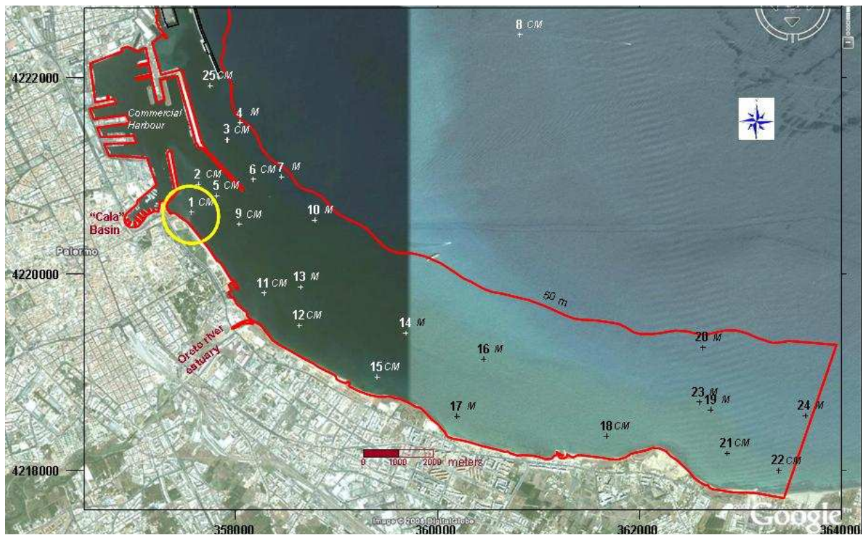
Figure 1: the distribution of the measuring stations (Porta Felice outfall is circled in yellow).
